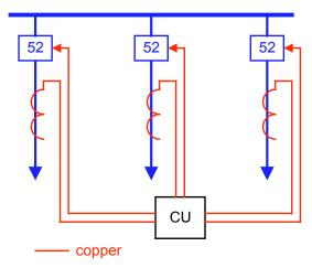
Fig.5. Centralized busbar protection.
