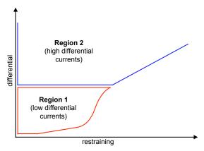
Fig.6. Two regions of the differential characteristic.
