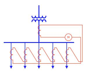
Fig.3. Busbar protection with linear couplers.
