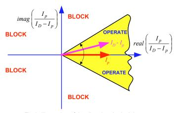
Fig.9. Illustration of the directional principle.
