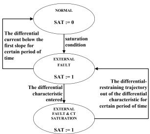
Fig.11. CT saturation detector: the state machine.
