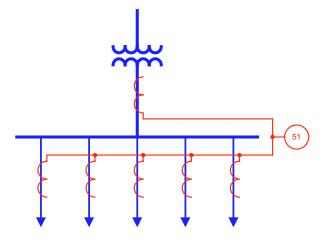
Fig.2. Overcurrent differential protection.
