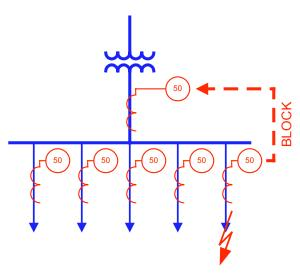
Fig.1. Illustration of the interlocking scheme.
