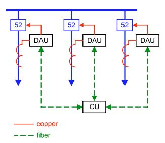
Fig.4. Distributed busbar protection.
