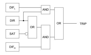
Fig.7. Adaptive trip logic.
