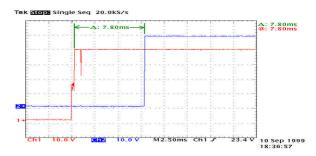
Figure 4: Digital input to digital output GOOSE timing.
