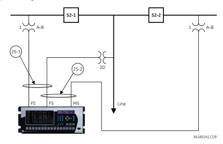
The steps to configuring the G30 for dual synchrocheck functions are the same as for example 1, with only some differences in the voltage input settings.
