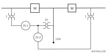
A second application is a small generation system that can operate in parallel with the utility source, or serve and maintain load separate from the utility source. In this application, it is typical to synchronize voltages across the load bus. This method requires synchrocheck from the generator to the load bus, and from the utility source to the load bus. Both synchrocheck functions use a common voltage measurement from the load bus.
