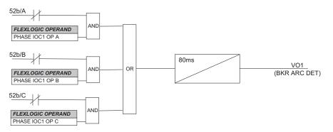
The timer should introduce a delay to avoid false signals due to a possible race between breaker auxiliary contacts operation and reset of the overcurrent elements. Virtual Output 1 can be used to send an alarm.
