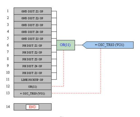
These diagrams show the FlexLogic<sup>TM</sup> equation as seen in Enervista UR Setup.
