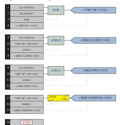
The FlexLogic<sup>™</sup> equations for this logic are shown below:
