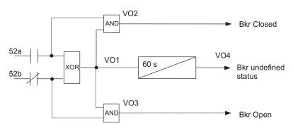
FIGURE 1. Breaker Status Monitoring Logic
