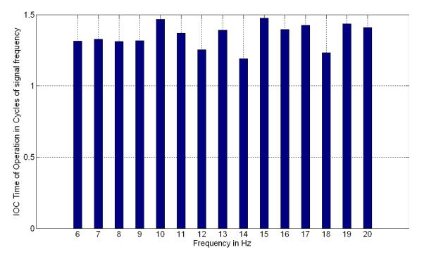
Figure 2: Time of operation of IOC at lower frequencies
