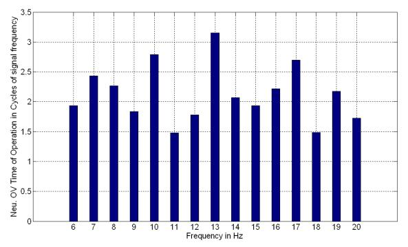
Figure 4: Time of operation of neutral overvoltage at lower frequencies
