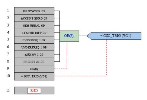
These diagrams show the FlexLogic<sup>TM</sup> equation as seen in Enervista UR Setup.
