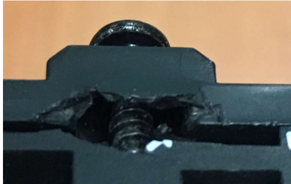
Fig. 9 Relay case damaged due to excessive screw tightening.
