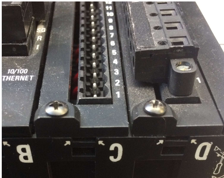
Fig. 7 Screws properly inserted.
