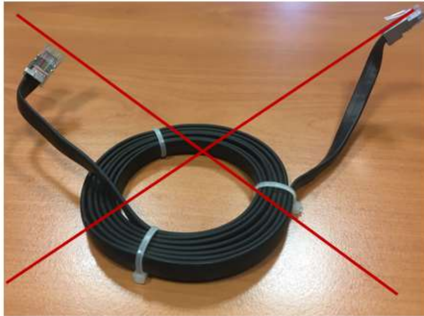
Fig. 24 Do not install longer cables that the ones needed.
