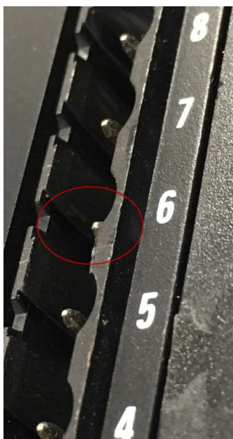
Fig. 6 Example of sagged pin.
