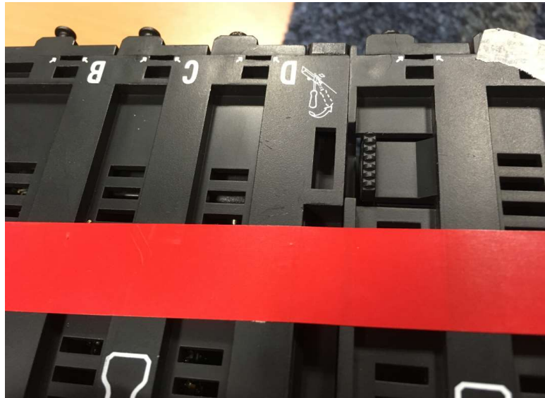
Fig. 15 Do not install self-adhesive tape covering case slots.
