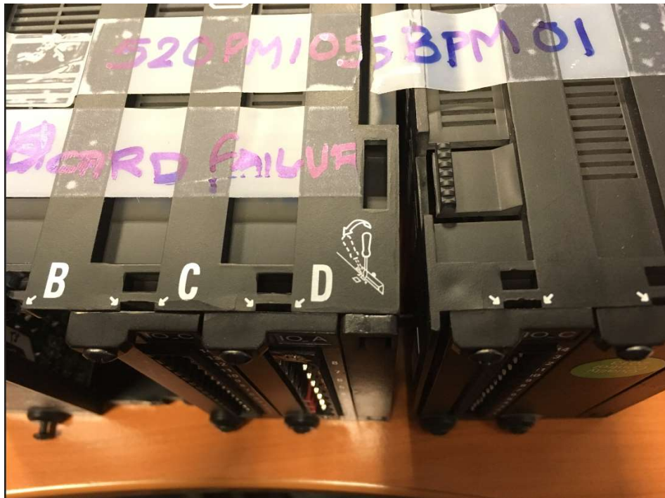
Fig. 13 Expansion module tabs damaged.
