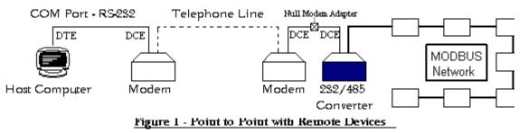
If multiple remote sites are required in point-to-point networks, then the above configuration must be duplicated for each site.
