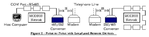
Remember that all devices, including the modems, must be configured to run at the same baud rate.
