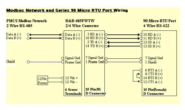
Note: The RTU port ground signal connection is not required but may be connected if needed. A 1-2 ft length should be enough for the 4 wire RTU cable (with 25 pin female and 15 pin male D connectors) between PLC and the 2/4 wire converter. Shield connection may not be important on such a small length. Only port 2 can be used for RTU communication on the 28 point Micro 90.
