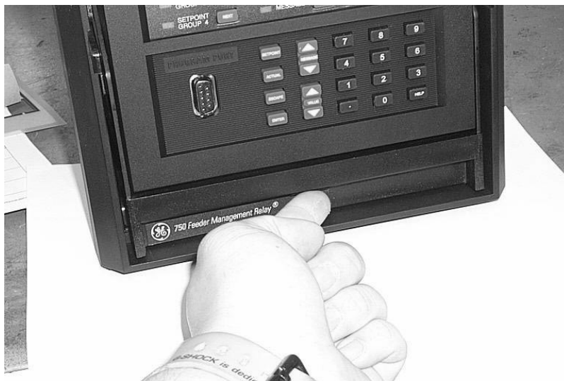
Figure 3-5: PRESS LATCH UP AND PULL HANDLE
