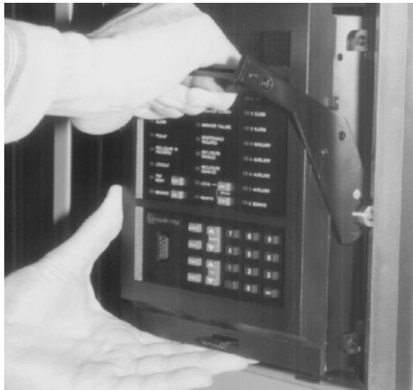
Figure 3–7: SLIDING THE UNIT OUT OF THE CASE
