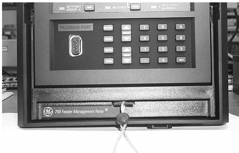
Figure 3-2: DRAWOUT CASE SEAL
