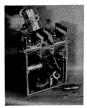
FIGURE 19 AF-400 Drive Converter Module with stud mounted SCRs showing removal of stud mounted SCR cell. 10-30 KVA, 230 or 460VAC
