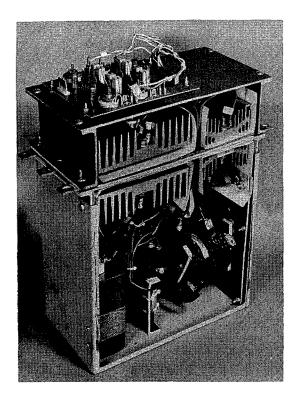
FIGURE 24 AF-400 Drive Inverter Phase Module 40-60 KVA, 460V AC standing on a table Press-Pak Main SCR cells stud mounted Commutating SCR cells. 3. After locating the defective Press-Pak Main SCR cell (1SP and 1SN) follow the instructions for Press-Pak Main SCR cells, 40-60 K.V.A, 230V AC units. See Figure 25.
