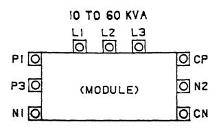
L1 to P1Checks positive phase 1 SCR, (1SP)L1 to N1Checks negative phase 1 SCR, (1SN)L2 to P1Checks positive phase 2 SCR, (2SP)L2 to N1Checks negative phase 2 SCR, (2SN)L3 to P1Checks positive phase 3 SCR, (3SP)L3 to N1Checks negative phase 3 SCR, (3SN)
