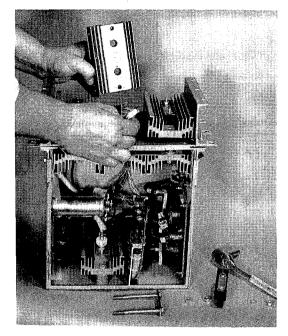
FIGURE 16 AF-400 Drive Converter Module showing removal of heatsink Press-Pak SCRs 40-60 KVA, 230 or 460V AC
