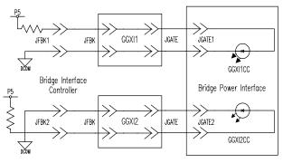
Figure 2. Board Identification Signals
