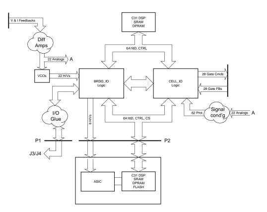
Figure 3. BICI Board Logic Architecture
