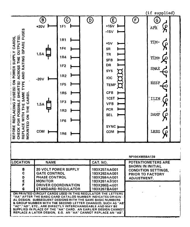
Figure 2-2 Location and Function of Driver-Regulator Cards
