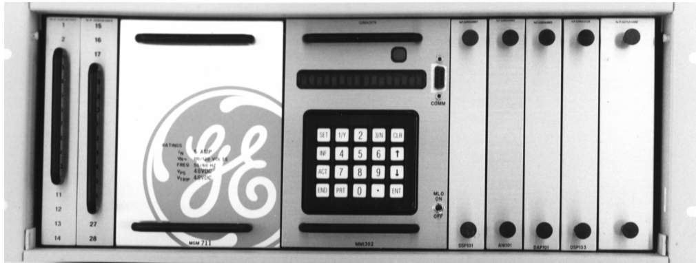
Figure 3-1. (8919475) Front panel of DLP1 Relaying System, showing keypad and test plugs.
