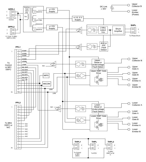
Figure 1. DSFC Board Block Diagram
