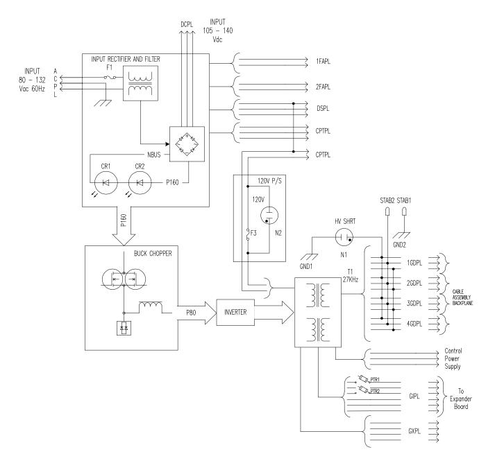
Figure 1. GDPA Board Block Diagram
