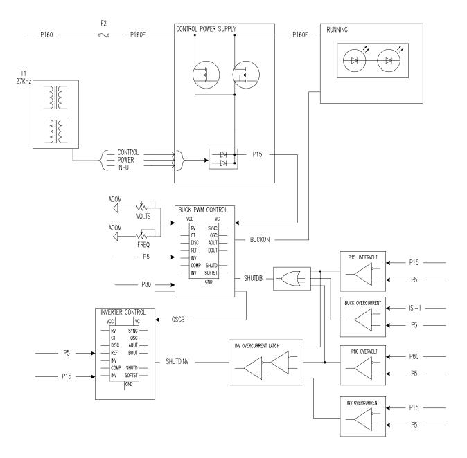
Figure 2. GDPA Board Control and Protection Block Diagram
