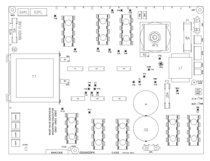
Figure 3. GDPA Board Layout Diagram
