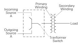
Figure 24. Schematic of the loop switch with ON-OFF radial switch.
