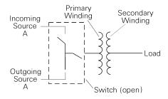
Figure 21. Schematic of the loop-radial switch.
