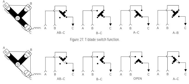
Figure 28. V-blade switch function.
