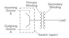
Figure 19. Schematic of the loop-feed switch.
