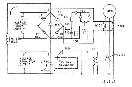
Figure 4. C.T. Forcing Unit Operation
