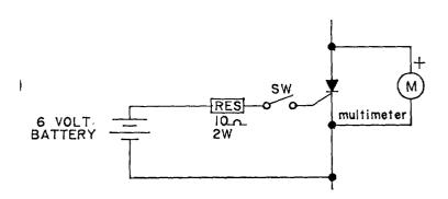
FIG. 24 SCR TEST CIRCUIT
