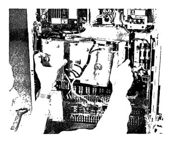
(Photo MG-5236-22) FIG. 27 REMOVAL OF CONVERSION MODULE
