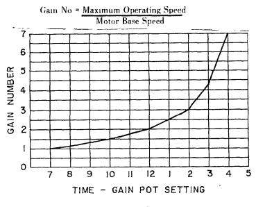
Time-Gain Pot Setting FIG. 23 GAIN ADJUSTMENT
