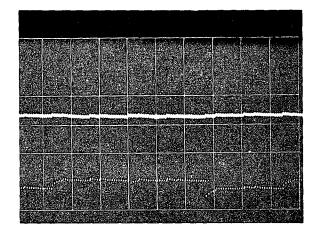
2 msec/div Normal l volt/division FIG. 19 PULSE OUTPUT (PO)
