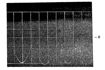
2 msec/div At low current level 1 volt/division FIG. 12 CURRENT FEEDBACK (CFB)
