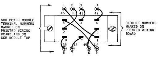
TOP VIEW - I. R. SCR MODULE WIRE CONNECTIONS
