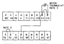
TERMINAL ARRANGEMENT ON 3SRC2000 REMOTE CONTROL STATION ADAPTER
