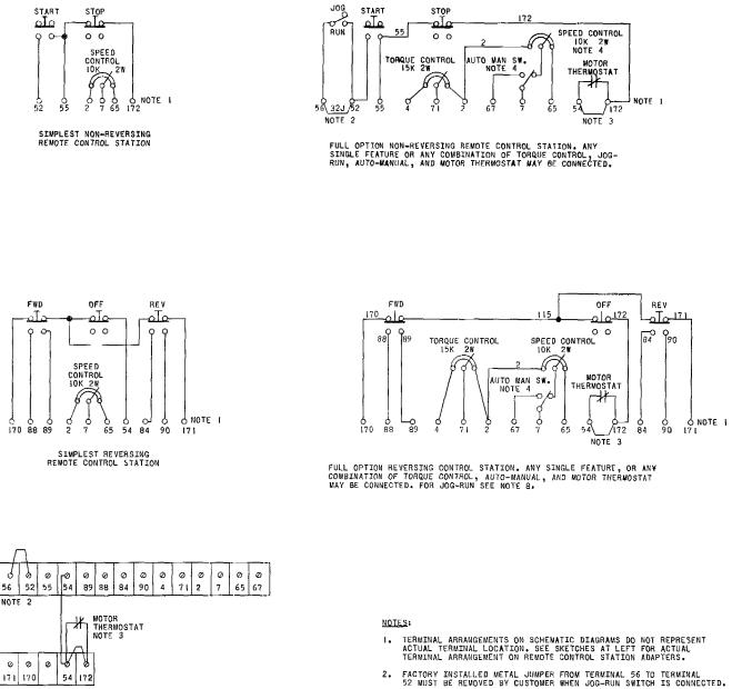
TERMINAL ARRANGEMENT ON 3SRC2001 REMOTE CONTROL STATION ADAPTER
