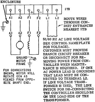
Figure 4. Power Wiring Connection Diagram
