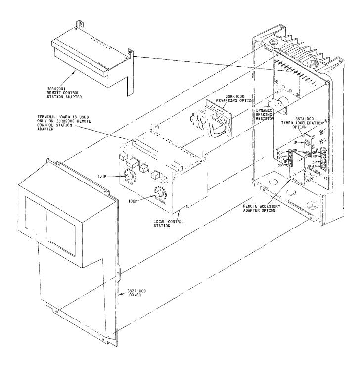
Figure 2. Exploded View Of Statotrol II Controller
