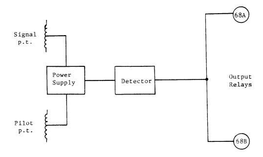
Figure 1. Voltage Balance Circuit
