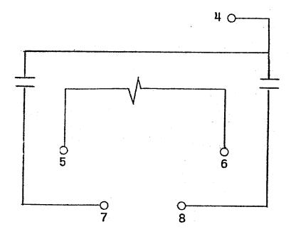
FIG. 1 (0257A5023-0) Internal Connections Diagram For Special Relay HAA99AA001
