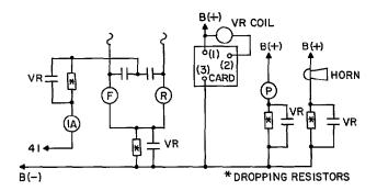
Fig. 2. Typical circuit for dual-voltage adapter
