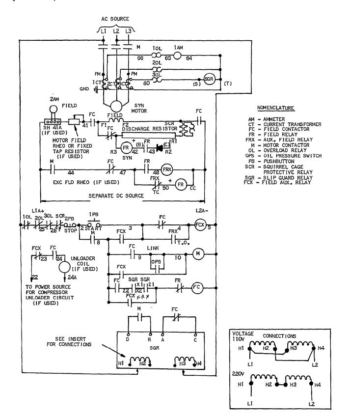
Typical Circuit for Synchronous Motor Control Showing Slip Guard Relay in Place of Magnetic Relay IC28201751
