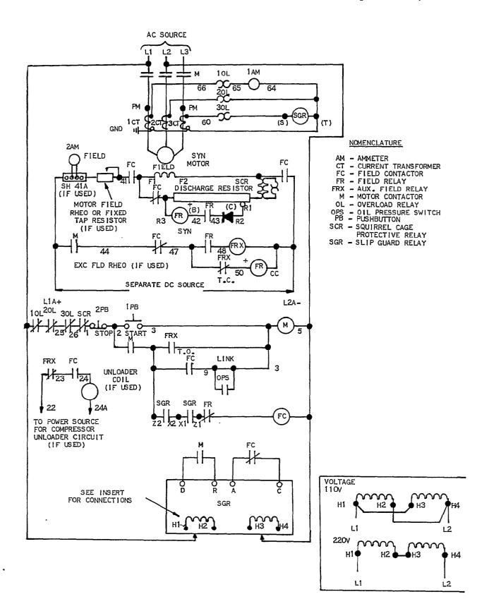
**Typical Circuit for Synchronous Motor Control**
