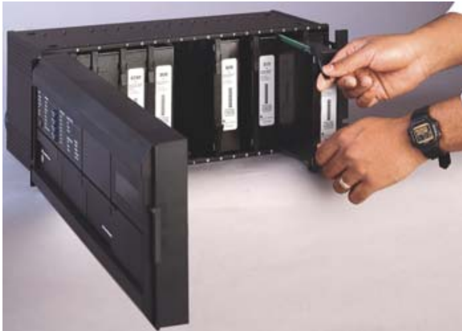
Figure 3-5: UR MODULE WITHDRAWAL/INSERTION
