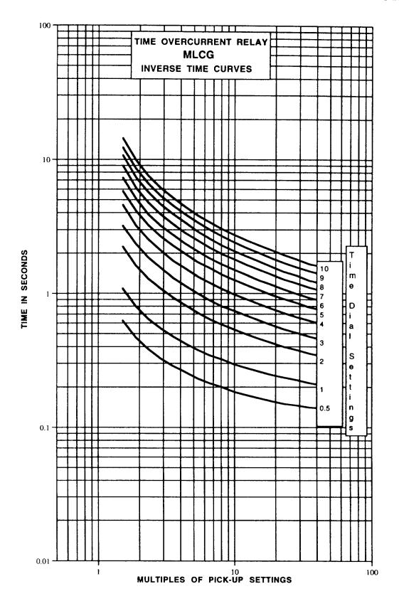
Figure 1 (GES-9873) TOC Inverse Time Characteristic Curve for the MLCG
