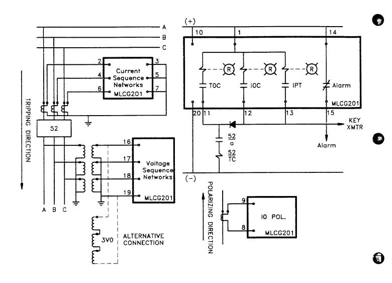
Figure 9 (0286A5304) Typical External Connections Diagram for MLCG
