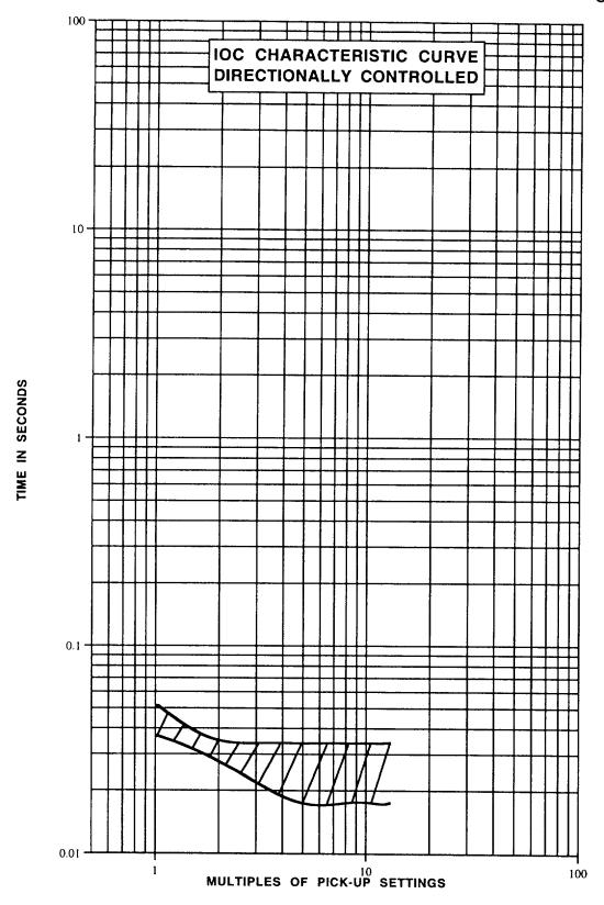
Figure 5 (GES-9877) IOC Characteristic Curve, Directionally Controlled, for the MLCG
