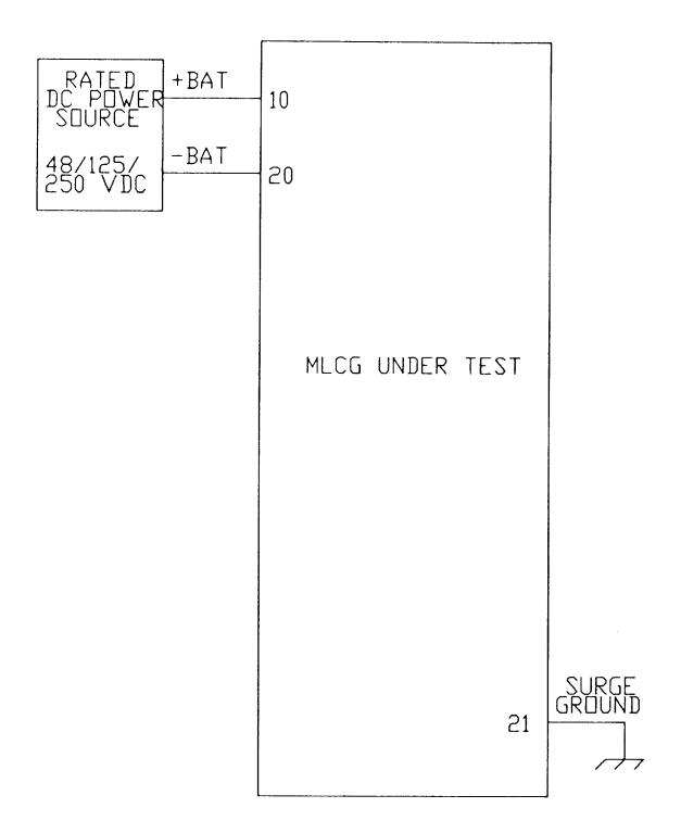
Figure 18 (0286A4931) Connections for Power Up Test and LED Test
