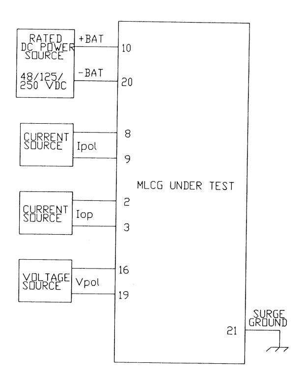
Figure 22 (0286A4935) Connections for Directional Tests, I and V Polarization
