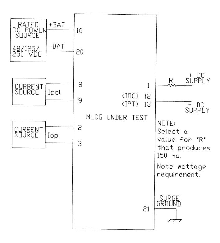
Figure 21 (0286A4934) Connections for IOC Tests and IPT Test
