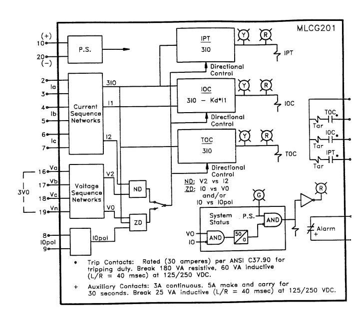
Figure 7 (0286A5303) Functional Block Diagram for MLCG
