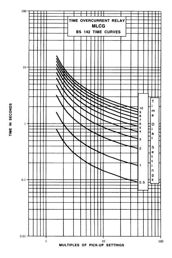
Figure 4 (GES-9876) BS142 Time Characteristic Curve for the MLCG
