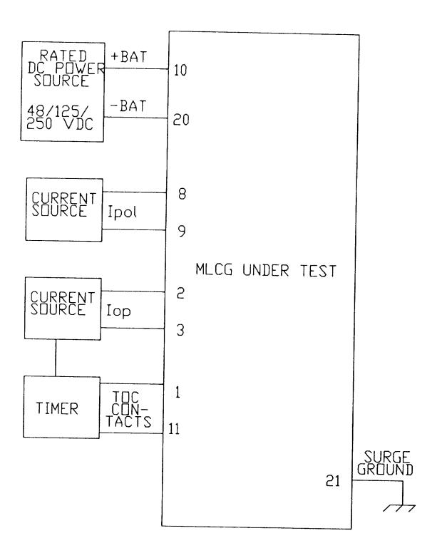
Figure 20 (0286A4933) Connections for TOC Time-Dial Test and TOC Definite-Time Test
