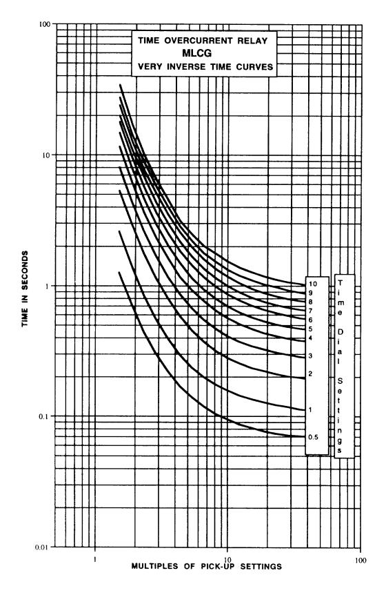
Figure 2 (GES-9874) TOC Very Inverse Time Characteristic Curve for the MLCG
