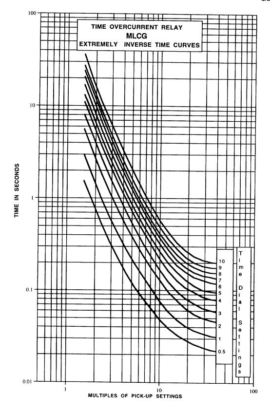
Figure 3 (GES-9875) TOC Extremely Inverse Time Characteristic Curve for the MLCG
