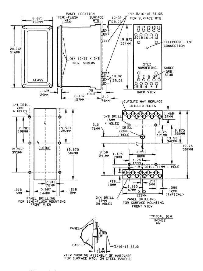
Figure 17 (0215B8430 [1]) Outline and Panel-Drilling Dimensions
