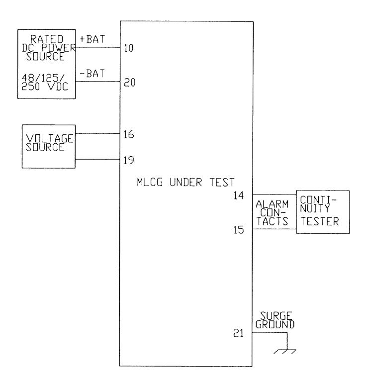
Figure 19 (0286A4932) Alarm Test Connections
