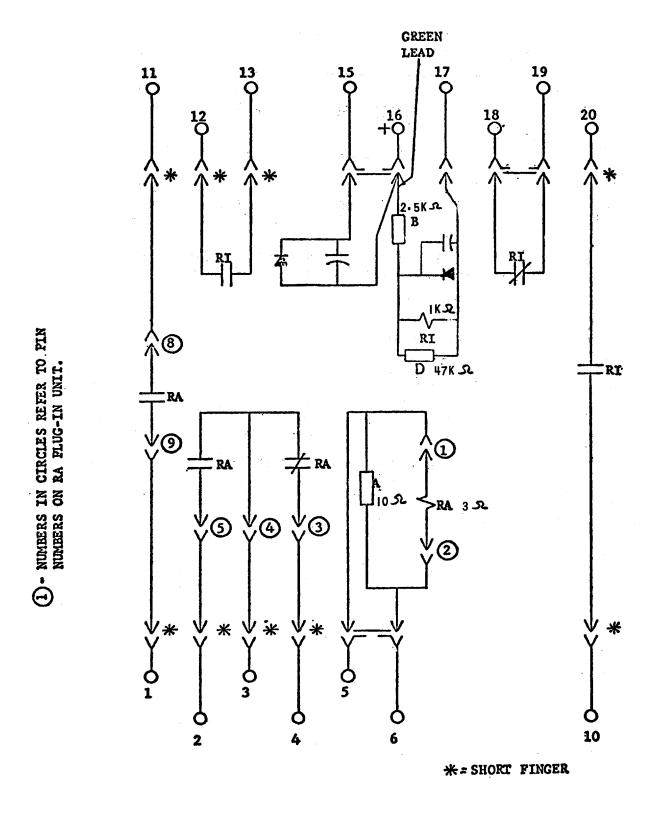
Figure 1 (0257A5087-0) INTERNAL CONNECTIONS FOR THE 12NAA99AB SPECIAL RELAY.
