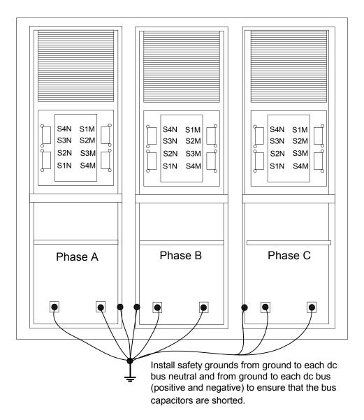
Figure 5. Dc Bus Safety Grounding
