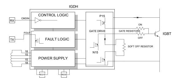
Figure 3. IGDH Subassembly Functional Block Diagram
