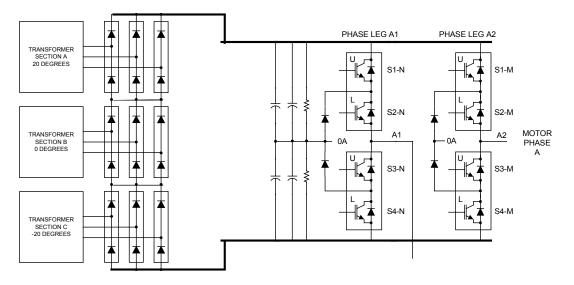
Figure 2. Power Converter Phase Diagram
