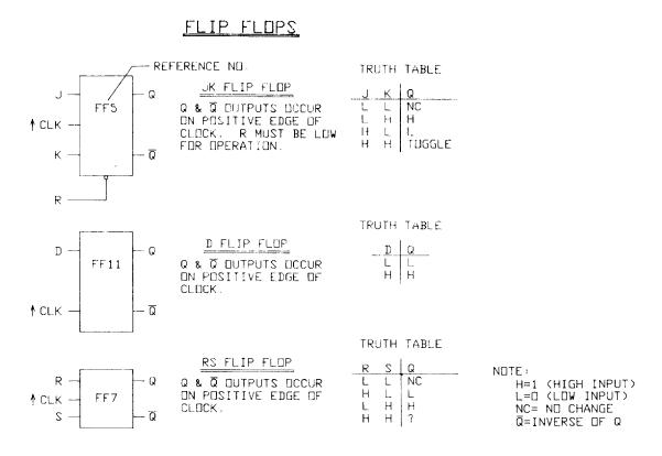
Figure SD-2 (0286A2775 Sh.2 [3]) Logic and Internal Diagram Legend
