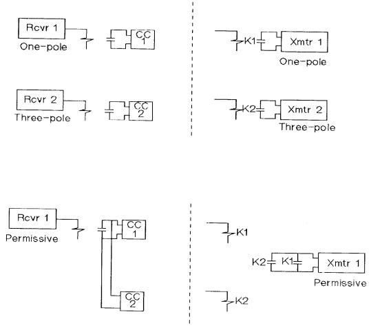
Figure CS-5 Connections for Communication Channels
