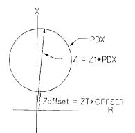
PDX has the characteristic shown in Figure CS-4. The reach of PDX is equal to PDX(Z1) where PDX is a reach multiplier and Z1 is the reach of the PD1 and ND functions.
