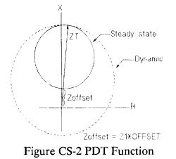
The PDT function can be set with a forward offset as shown in Figure CS-2 to the left, and the response of the function can be controlled via a time constant setting. Both of these features are used to minimize the effects of load flow.
