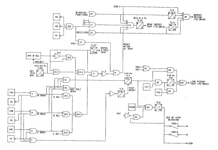
Figure SD-7 (0179C8269 Sh.3 [1]) Weak Infeed/Repeat Key/Line PU/Out of Step
