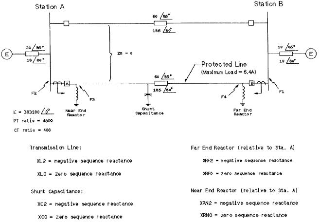
Figure CS-1 Sample Power System
