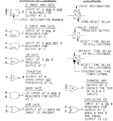
Figure SD-2 (0286A2775 Sh.1 [3]) Logic and Internal Diagram Legend
