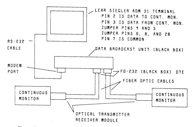
Figure CM-4 (0285A9837 [1]) Connection for Multiple Continuous Monitors
