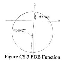
The blocking function has the characteristic shape shown to in Figure CS-3. The offset is equal to the forward offset in the PDT function and the reach of the function is a multiple (PDB) of the forward reach (ZT) of the PDT function (see Figure CS-2).
