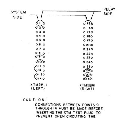
Figure HD-5 (0285A9896) XTM Connections for Dir. Ck. (Non-Trip Direction)
