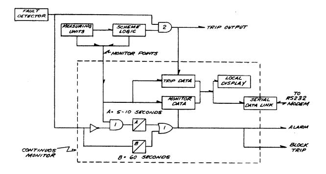
Figure CM-1 (0285A9897) Simplified Functional Diagram Depicting Continuous Monitor Operation
