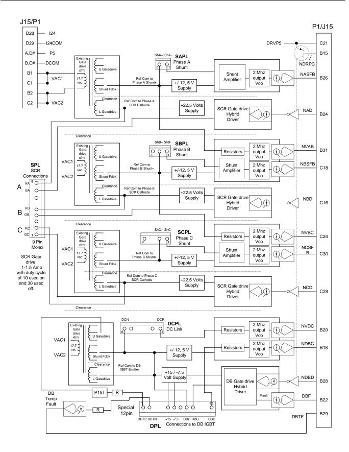
Figure 1. SCNV Board Block Diagram
