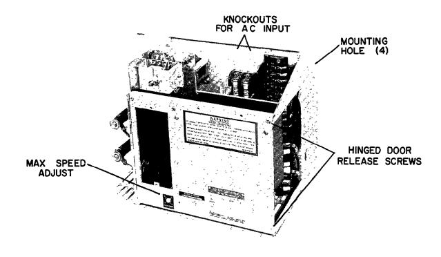
POWER UNIT ASSEMBLY – LESS ENCLOSURE Figure 1
