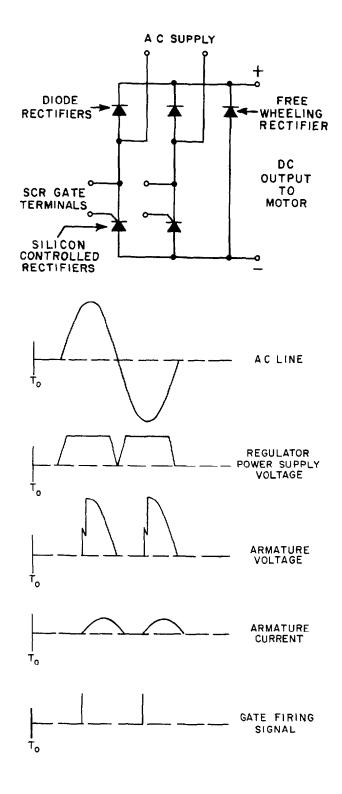
Figure 6 Typical Waveforms
