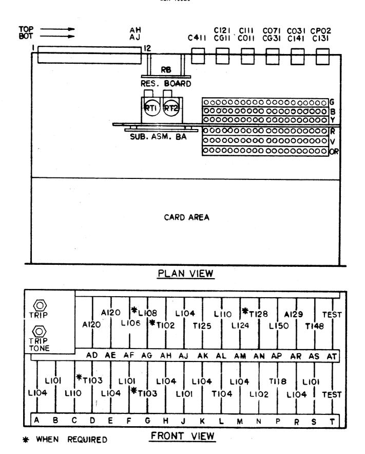
Fig. 3 (0273A9118-0) Component Locations for the Type SLA54F Relay
