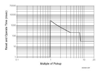
Figure 5-19: COMPOSITE RECLOSER CURVE WITH HCT ENABLED
