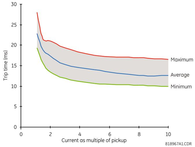
Figure 5: Operating speed of short-circuit protection – SR750 and reference
