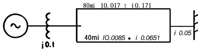
Fig. 7. Electrical system model
