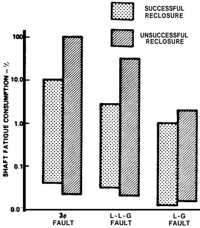
Fig. 5. Ranges of shaft fatigue duty (single incident)
