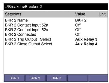
Once programmed in the breakers menu, the Trip outputs are defaulted to "Operate" in the menu of any protection element upon "Trip" function selection. One can easily deselect the trip outputs for the breakers which do not need to trip during operation. If "Alarm" or "Configurable" function is selected for the element, the selected trip outputs will automatically revert to "Do Not Operate".
