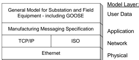
Figure 1: UCA substation profile.
