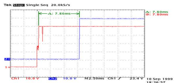
Figure 4: Digital input to digital output GOOSE timing.
