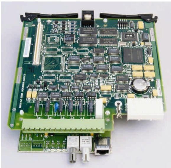
Figure 2: Modular CPU with fiber Ethernet Port(s).
