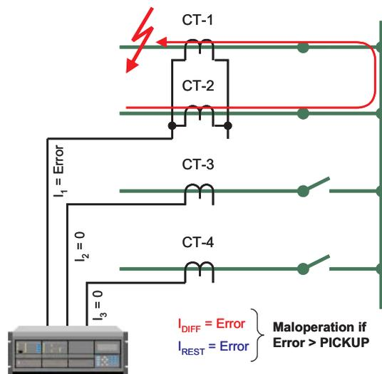
FIGURE 1. Sample System with Two CTs Paralleled
