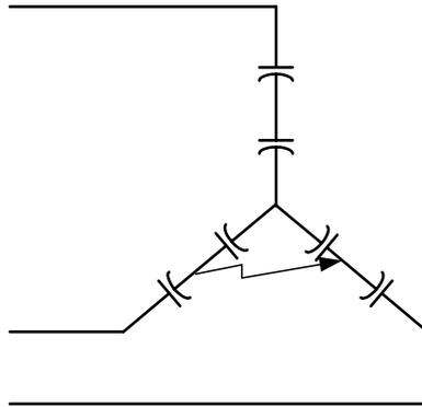
Fig. 17 – Mid-rack Fault
