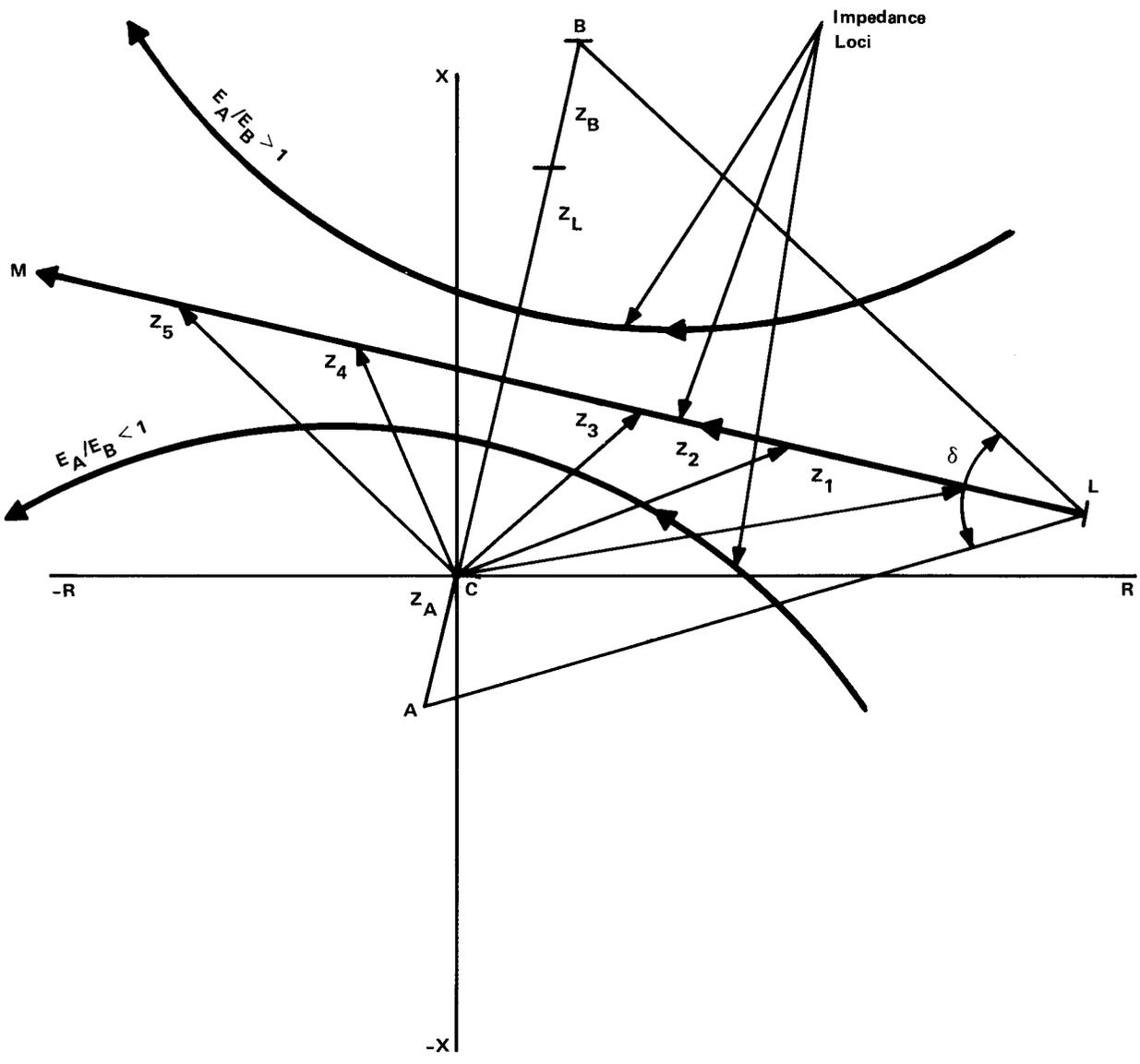
$\delta = \text{Angle of Separation Between Systems}$
