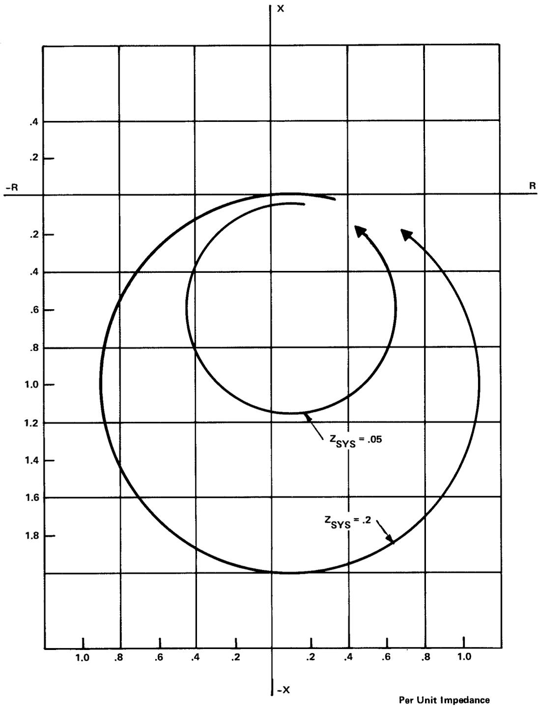
Fig. 3. Loss of synchronism characteristic for tandem compound generator – voltage regulator in service
