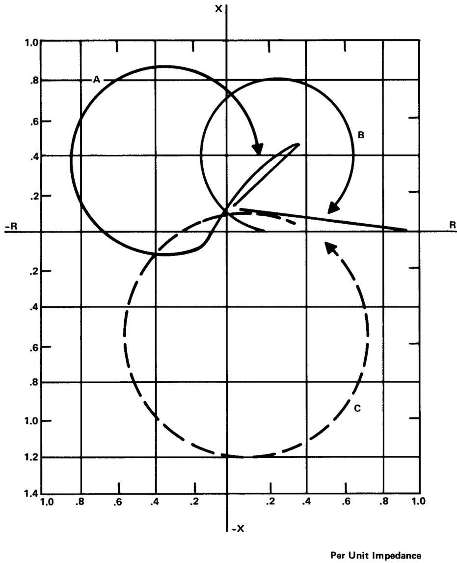
Fig. 5. Loss of synchronism characteristic — cross compound generator —  $Z_{SYS} = .2$  to  $.4$
