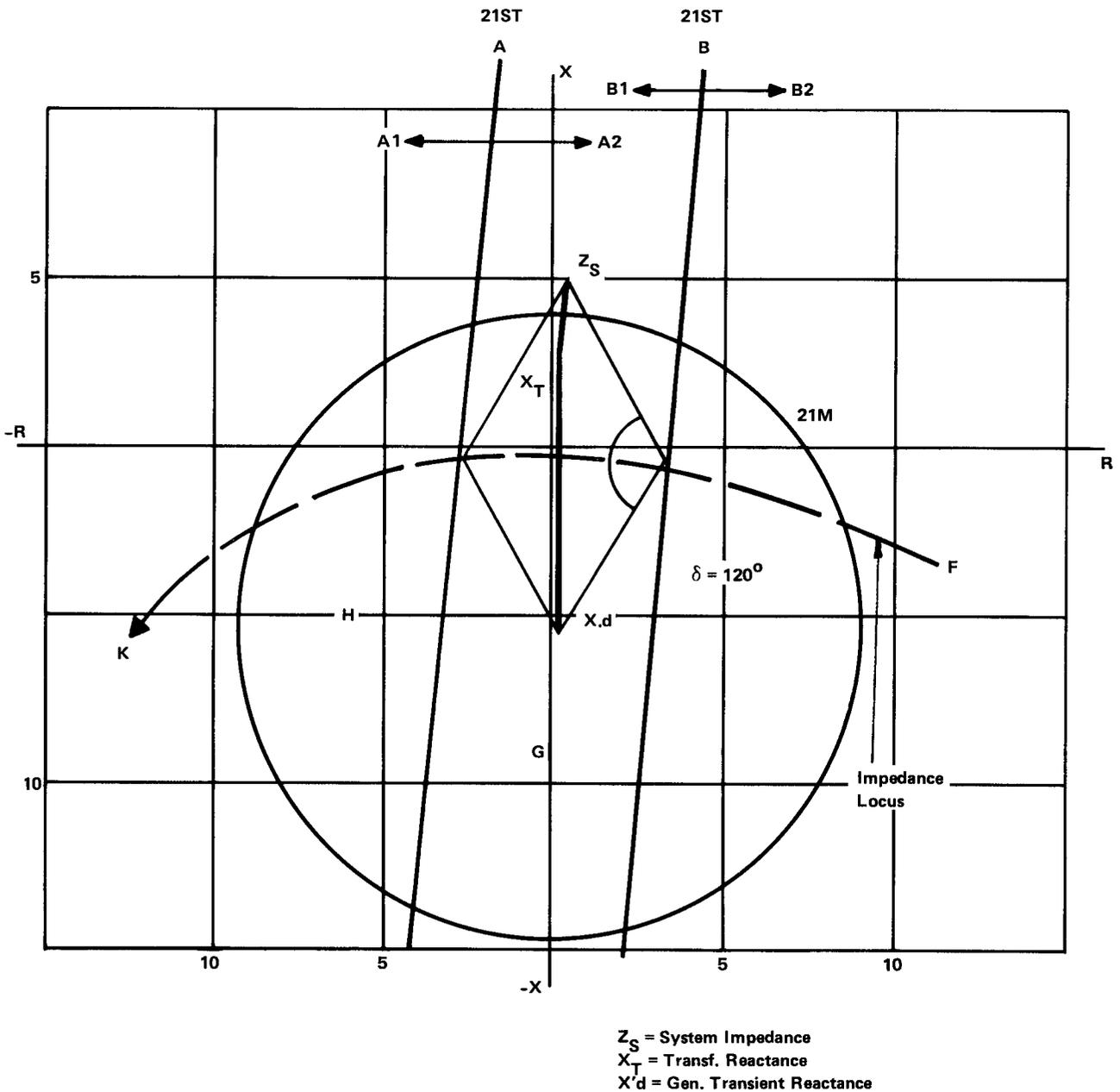
Fig. 6. CEX – CEB blinder out of step relaying scheme
