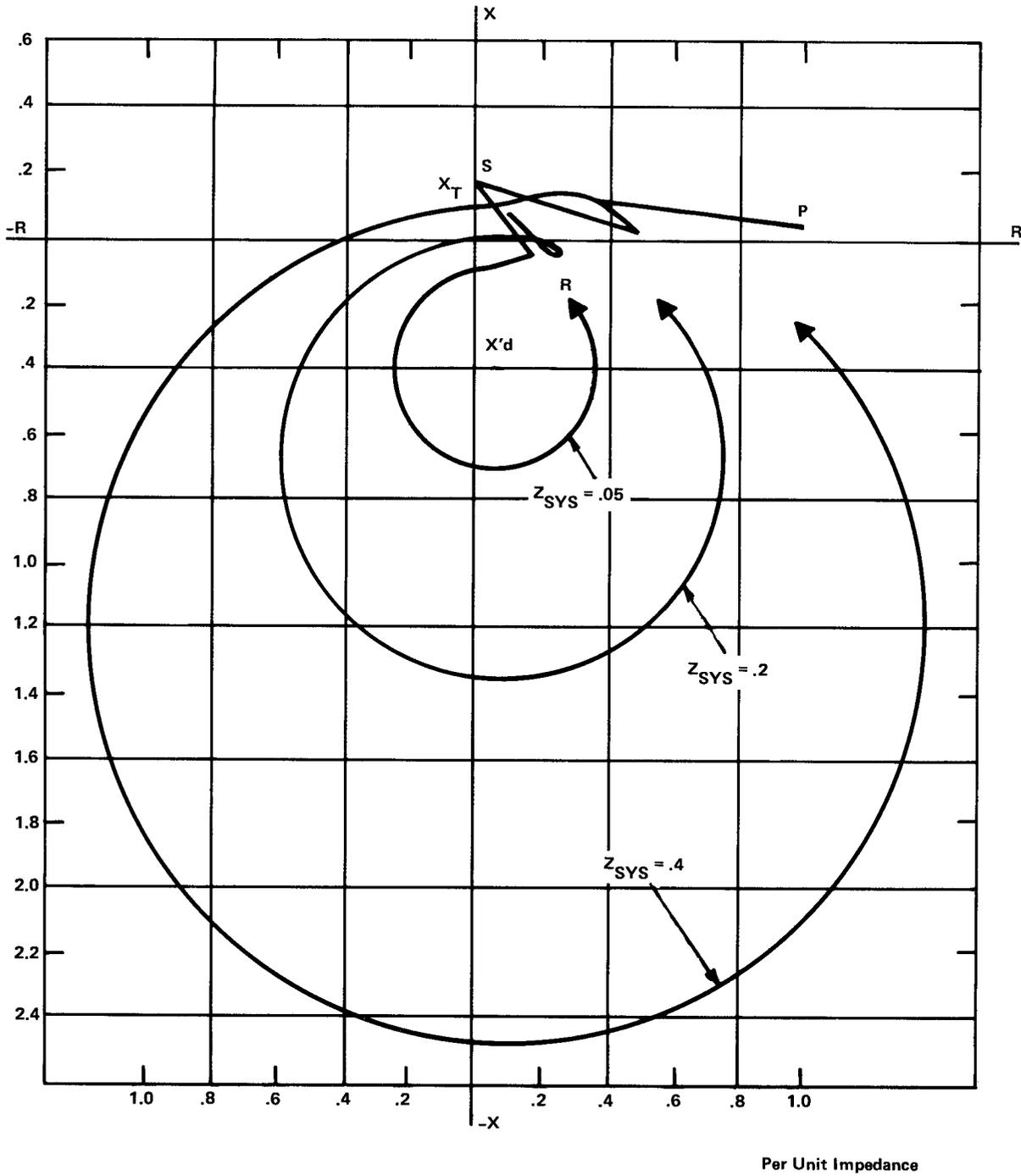
Fig. 2. Loss of synchronism for a tandem compound generator – voltage regulator out of service
