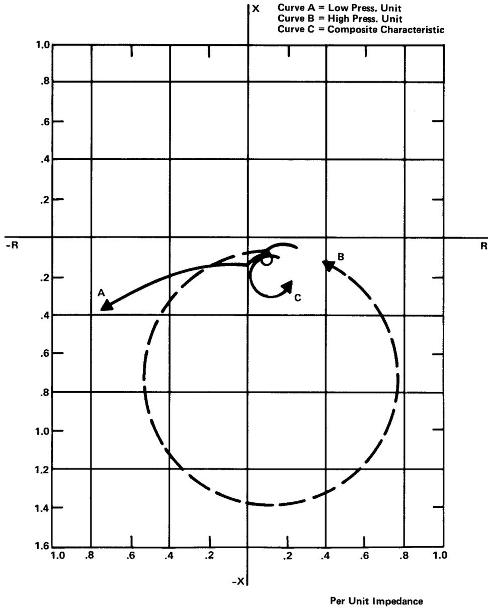
Fig. 4. Loss of synchronism characteristic — cross compound generator —  $Z_{SYS} = .05$
