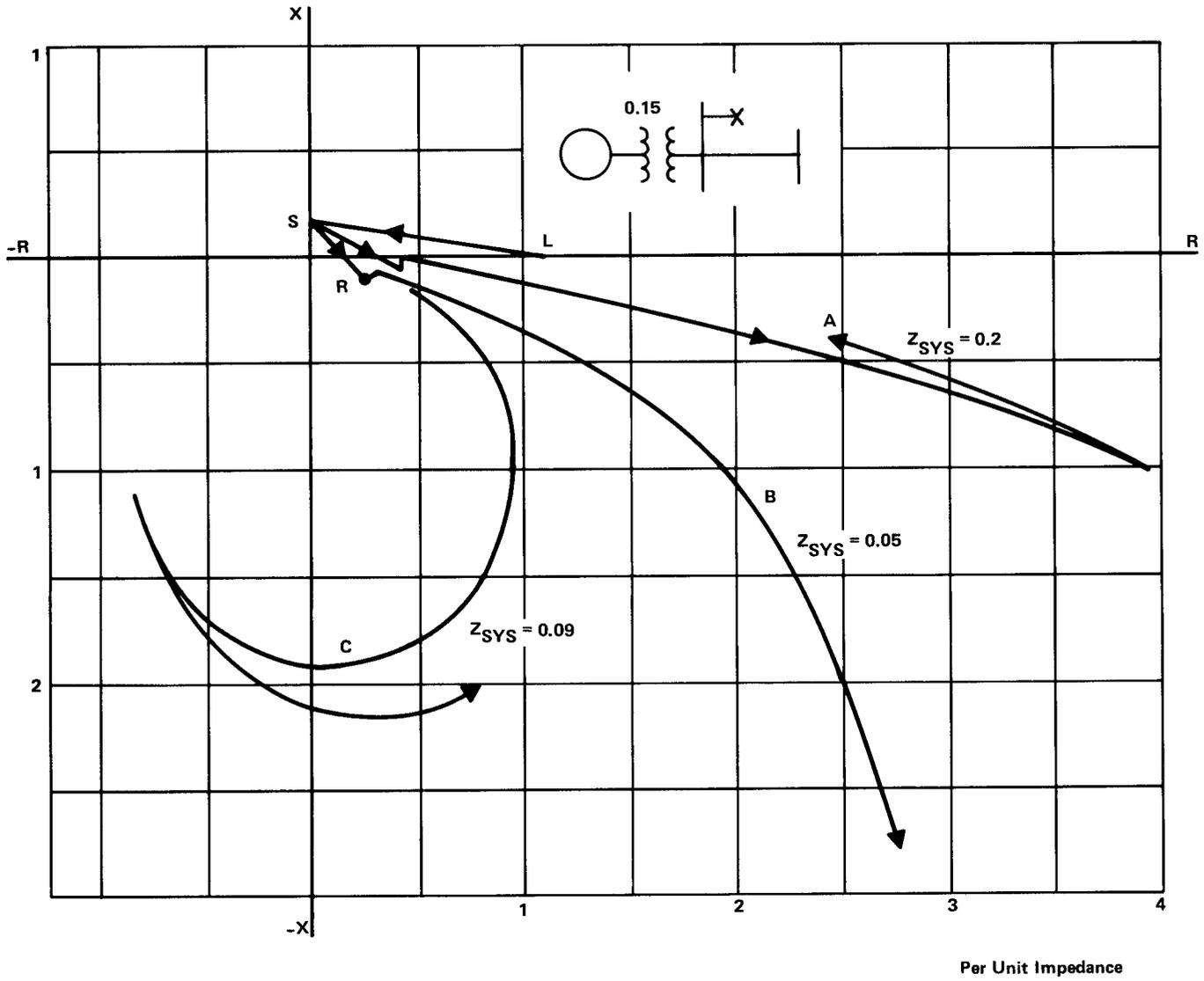
Fig. 9. Stable transient swings – tandem compound generator
