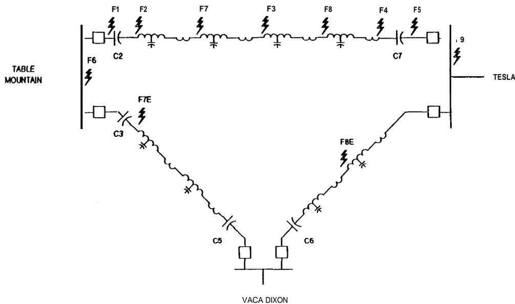
Figure 3: Series Compensated MPS System
