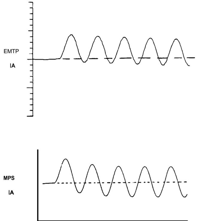
Figure 10: Fully Offset Current Waveforms
