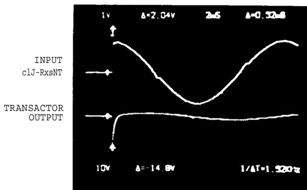
*Figure 10:* TYS Transactor Response for Step Change in Current
