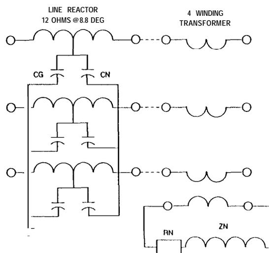
Figure 1: Typical MPS Line Section
