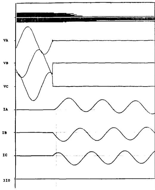
Figure 6: Model Power System Output 3 Phase Fault
