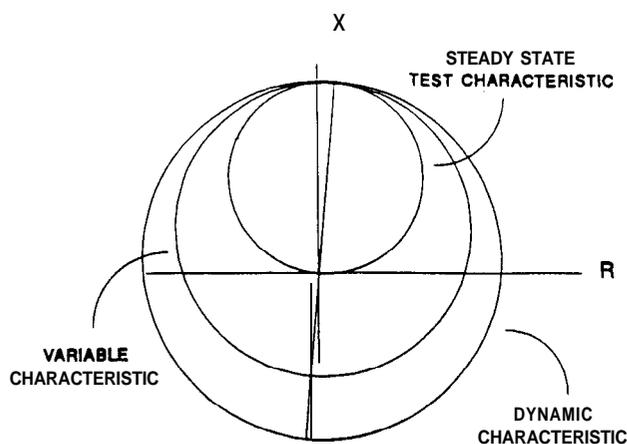
*Figure 1: Typical Dynamic, Variable, and Steady State Mho Characteristics*
