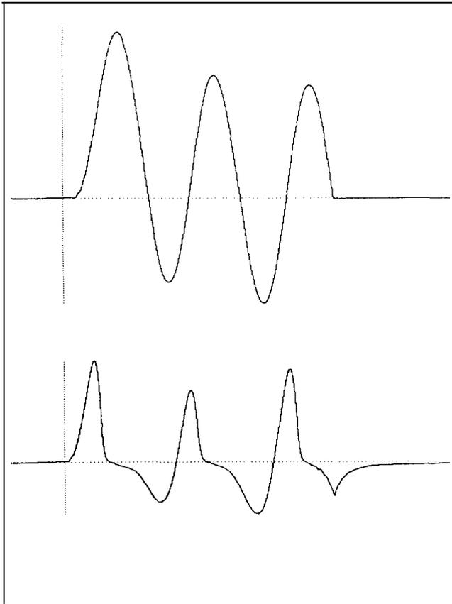
**Figure 12: Example of CT Saturation on the MPS**
