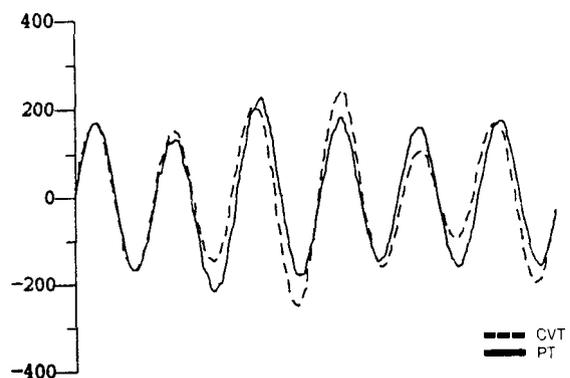
**Figure 14: EMTP PT and CVT Voltages for Series Compensated System**
