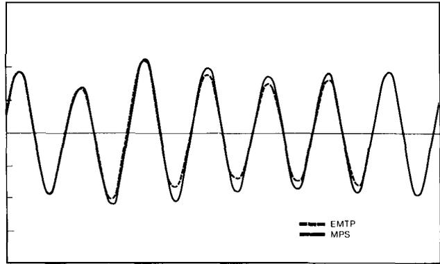
**Figure 13: EMTP and MPS PT Voltages for Series Compensated System**
