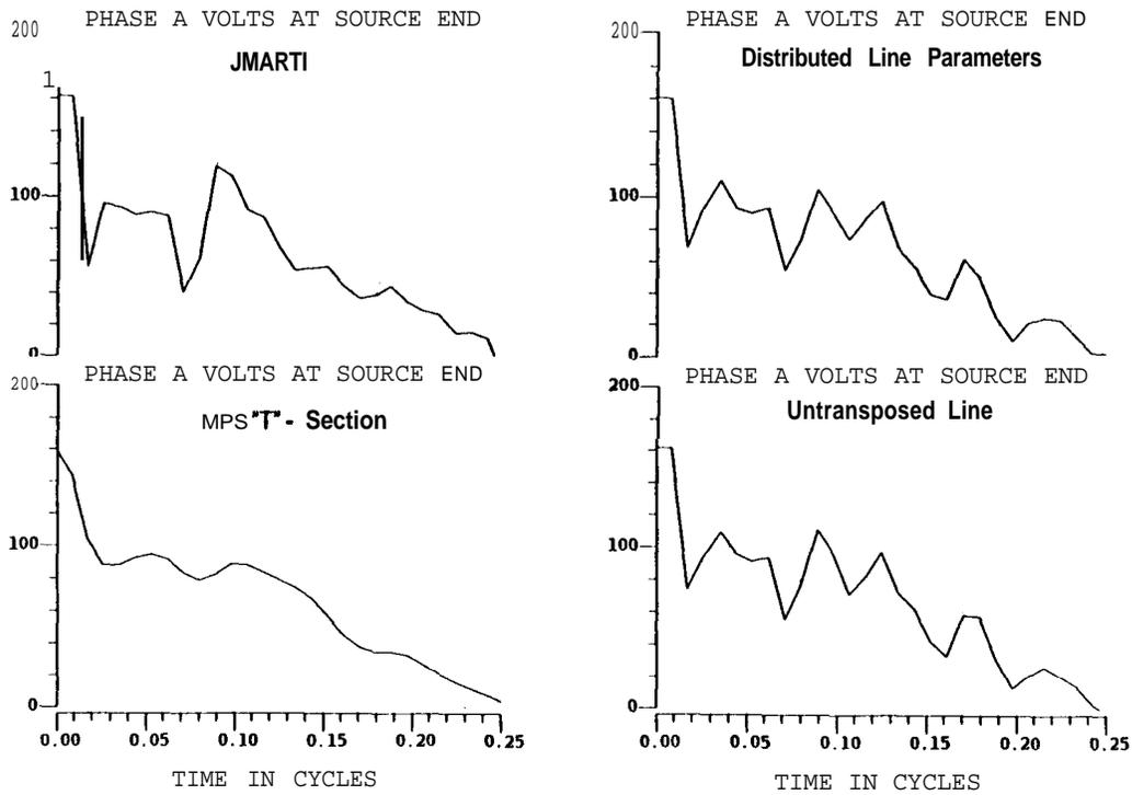
Figure 5: EMTP PT Voltage Waveforms - Expanded
