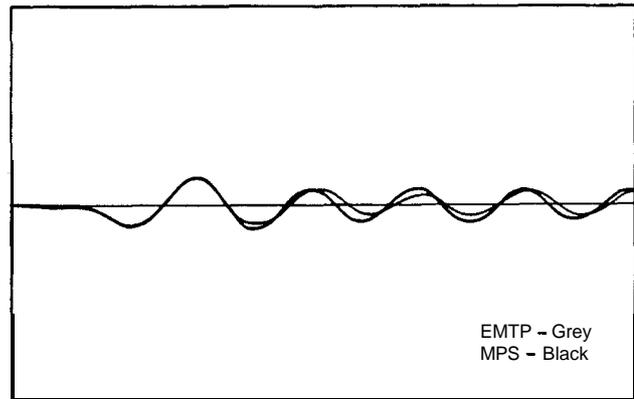
*Figure 16:* EMTP and MPS Fault Currents for Series Compensated System
