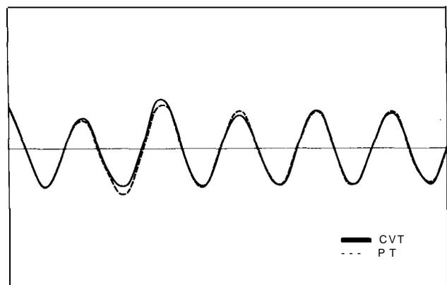
**Figure 15: MPS PT and CVT Voltages for Series Compensated System**
