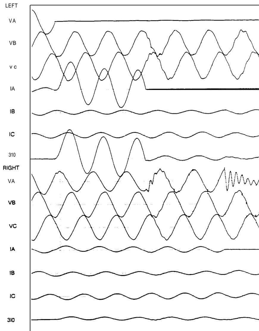
Figure 17: Currents and Voltages for MPS Single Pole Trip
