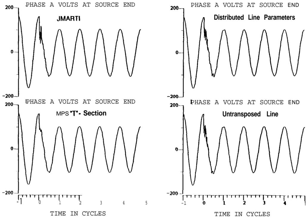
Figure 4: EMTP PT Voltage Waveforms for Four Line Models
