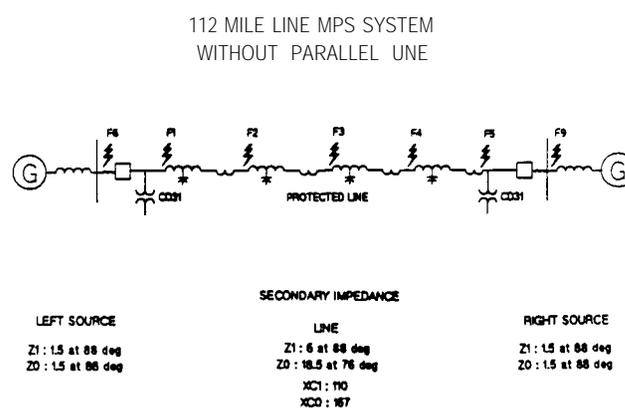
Figure 2: Typical Transmission Line
