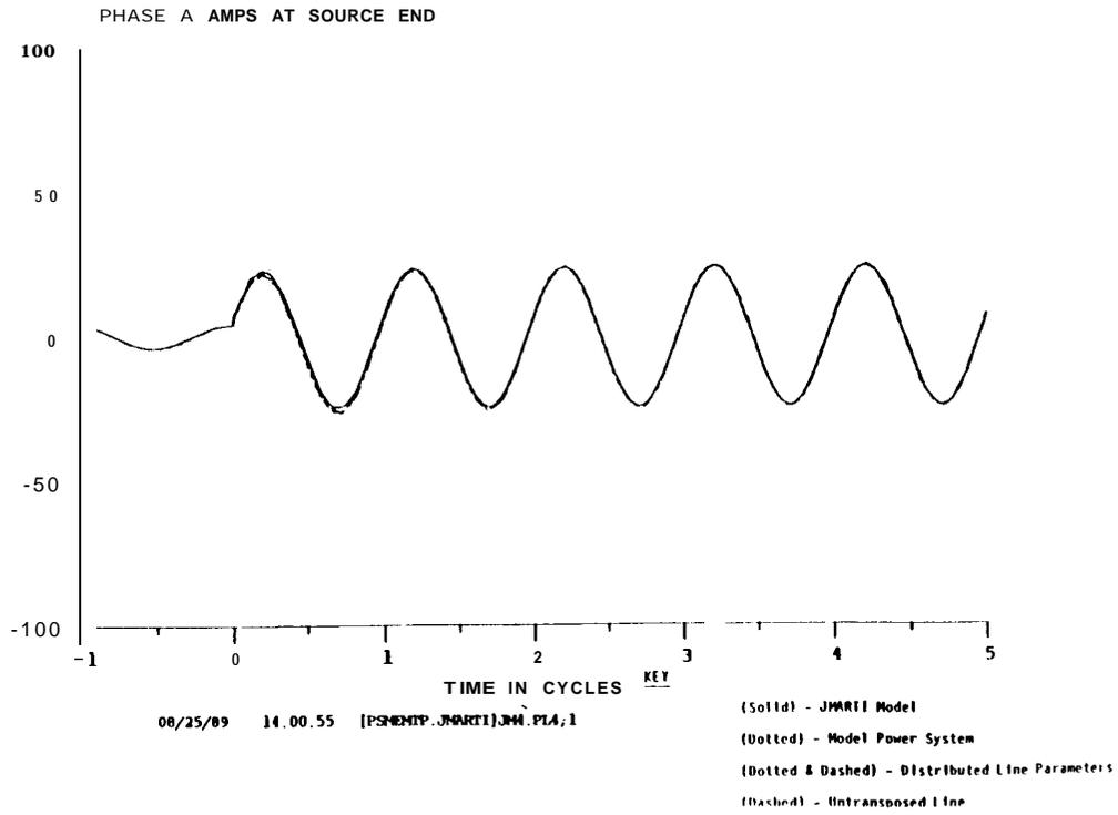
Figure 8: Composite EMTP Current Waveforms
