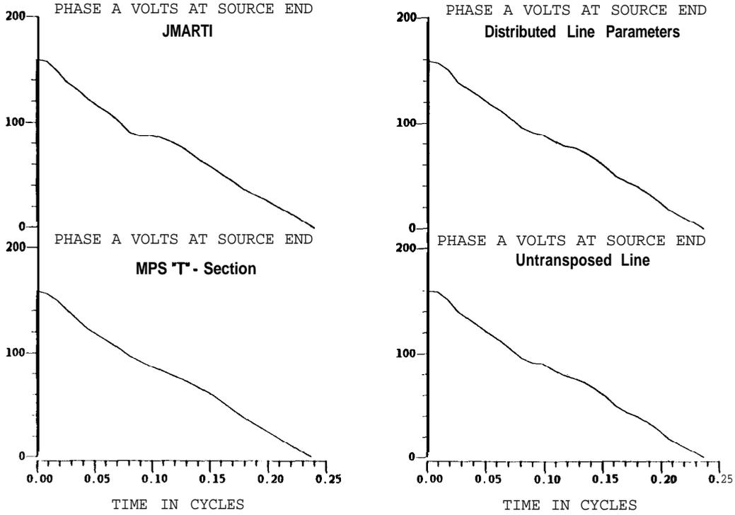
Figure 6: EMTP CVT Voltage Waveforms - Expanded
