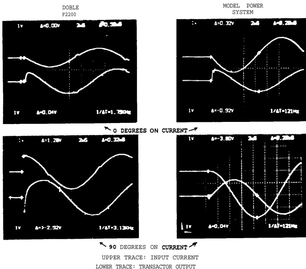
Figure 7: TYS Transactor Output Voltage
