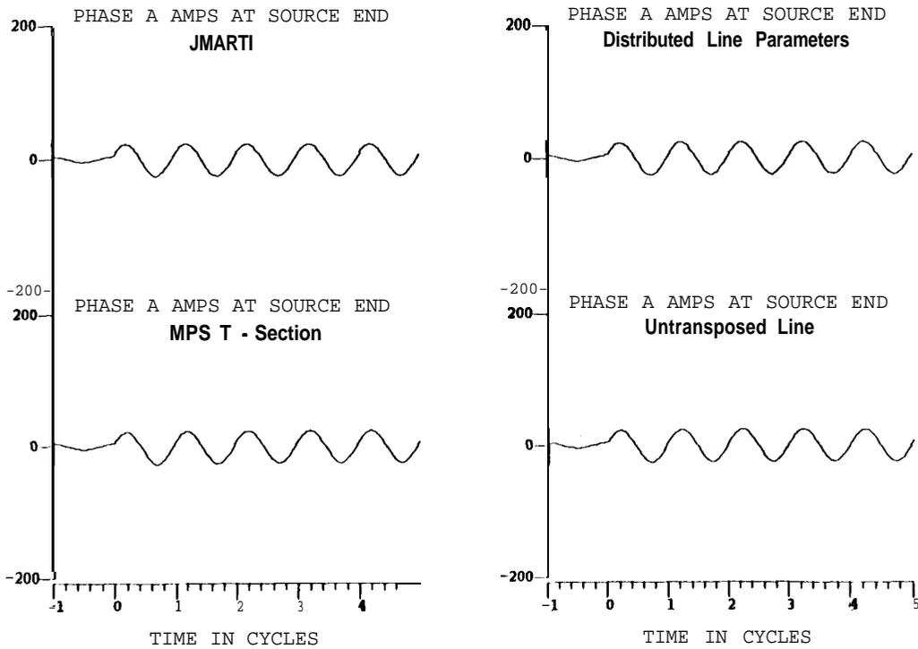
Figure 7: EMTP Current Waveforms for Four Line Models
