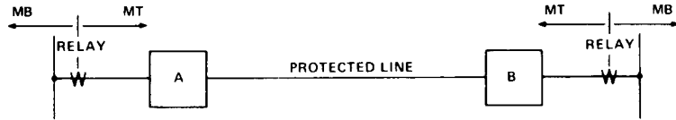
Figure 8. Mho Supervised Phase Comparison Blocking Scheme
