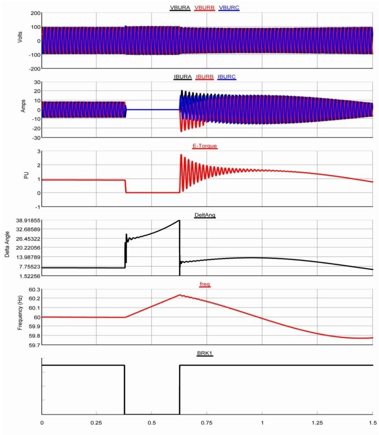
Fig. 2 RTDS simulation of Aurora vulnerability.
