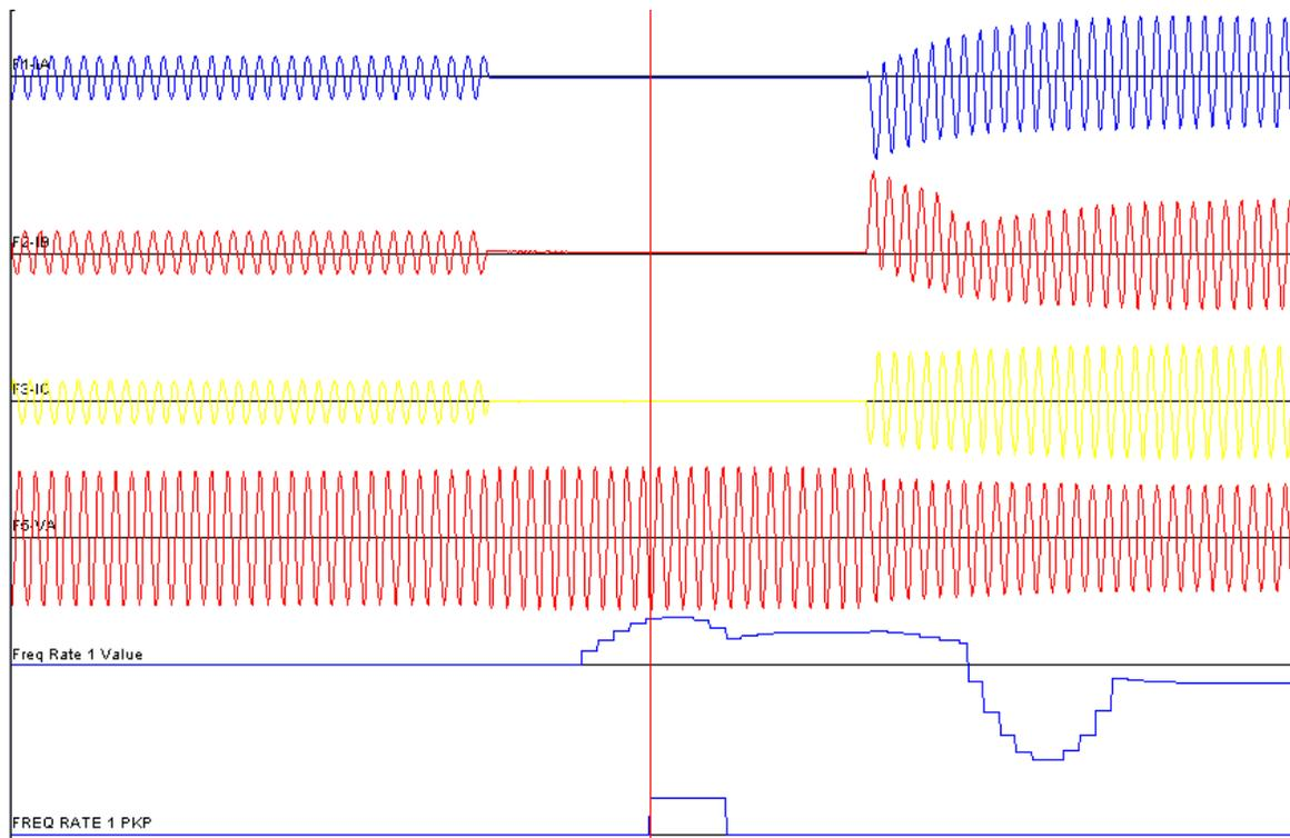
Fig. 3 Testing of ROCOF element of UR G60 during aurora vulnerability.
