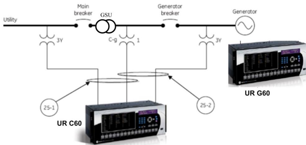
Fig. 4 Implementation of additional security with UR C60 for synchronism-check.
