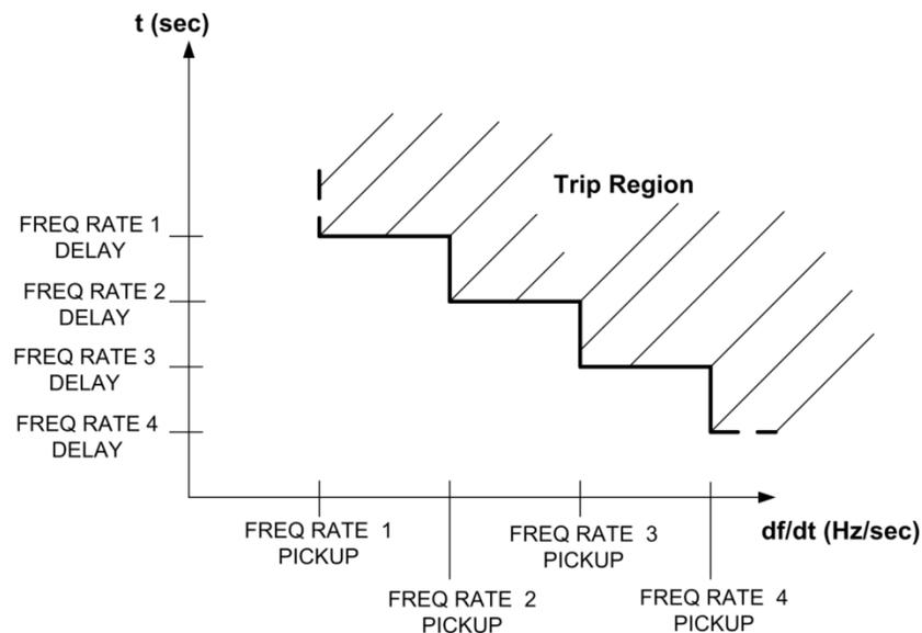
Fig. 1 consolidated characteristic using four ROCOF elements of UR G60.
