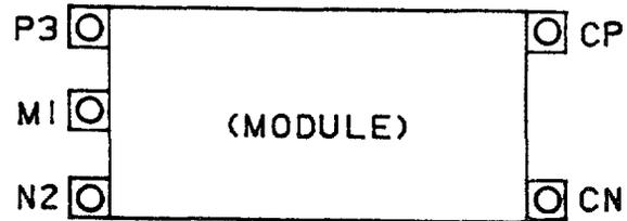
P3 to M1 Checks positive inverter SCR and diodes.
