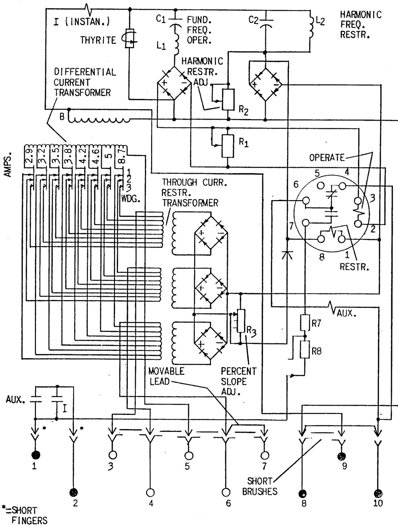
Fig. 11 Internal Connections of Type BDD16B Relay
