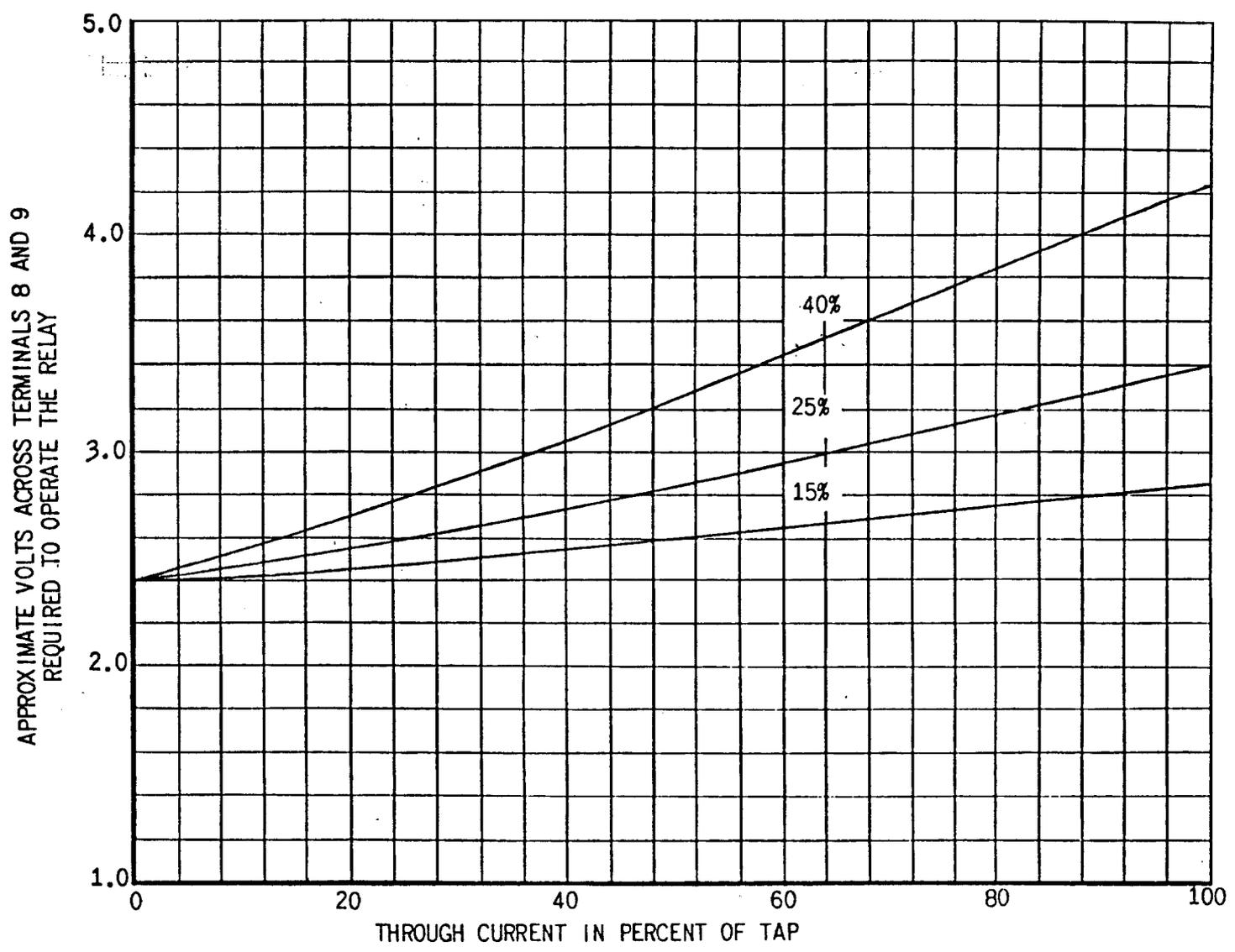
Fig. 15 Differential Voltage Operating Characteristics of Type BDD Relay
