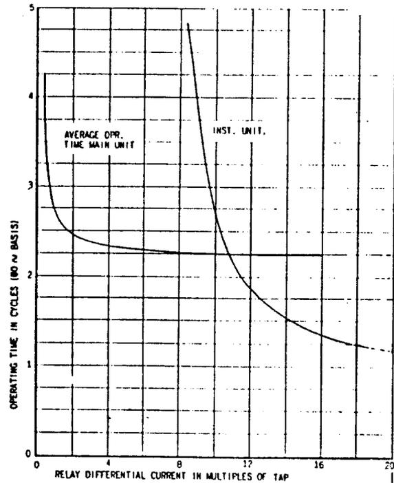
Fig. 1 Operating Characteristics of Type BDD Relay
