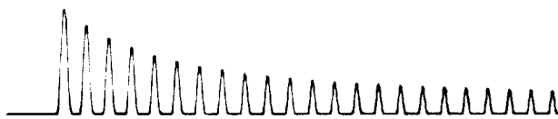
TYPICAL TRANSFORMER MAGNETIZING INRUSH CURRENT WAVE
