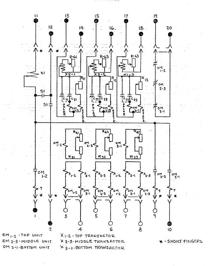
Fig. 1 (0165A6054-1) Internal Connections Diagram for the 12 CEB99AC(-) A Relay
