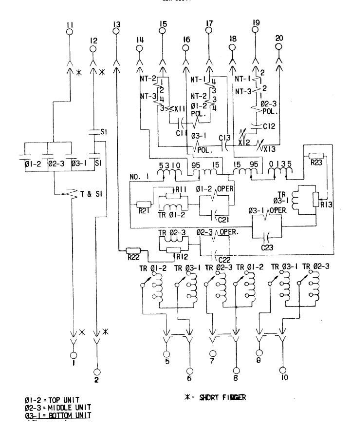
FIG. I (0227A7013-0) Internal Connections Diagram For The CEY51B Relay (Front View)
